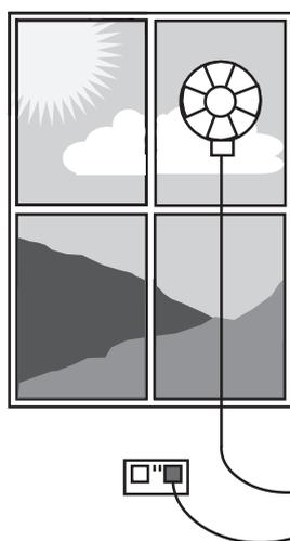
A Cool Control thermostat being used to control the temperature of a room by activating an extractor fan (max 300W). Site the probe within one of the cages to be protected. Choose either one high up or the one containing the least heat tolerant animal. Set the temperature to about 5° below the maximum permitted.
