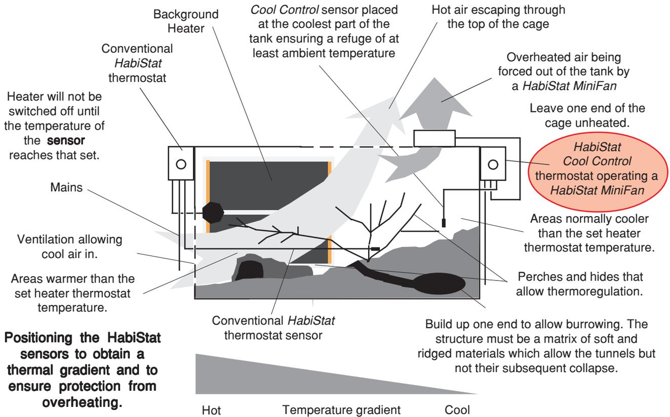
**Positioning the HabiStat sensors to obtain a thermal gradient and to ensure protection from overheating.**
